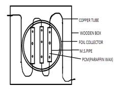
Fig:3.1 Experimental Set up of Solar Water Heater with PCM
